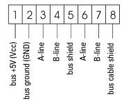
**Note:** To daisy-chain devices, connect both the outgoing and the incoming wires to terminals 3 and 4. Then if you have to remove the connector, the bus will still be active.
