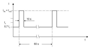
Figure 4-24 S6 duty cycle with initial load for a duty cycle duration of 60 s
