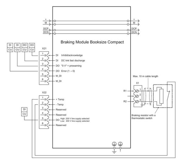
Figure 6-8 Connection example for Braking Module Booksize Compact and braking resistor with a thermostatic switch
