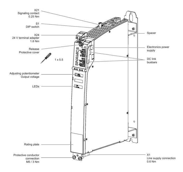
Figure 8-1 Interface overview, Control Supply Module
