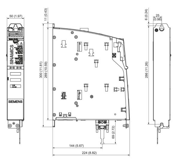
Figure 6-9 Dimension drawing of Braking Module Booksize Compact, all dimensions in mm and (inches)
