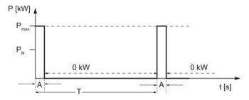
Figure 6-5 Duty cycle for braking resistors without a thermostatic switch
