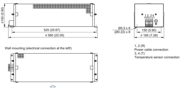
Figure 7-3 Dimension and installation drawing (roof and wall mounting) of braking resistor 6SE7018-0ES87-2DC0 where  $P_n/P_{max} = 1.25 \text{ kW}/7.5 \text{ kW}$ , all dimensions in mm and (inches)
