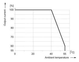
Figure 4-25 Output current as a function of the ambient temperature
