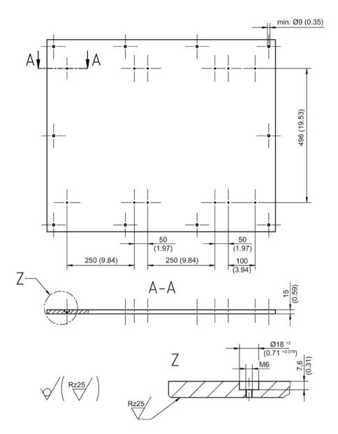
Figure 4-10 Drilling pattern for the High Frequency Drive without Active Line Module booksize, all data in mm and (inches)
