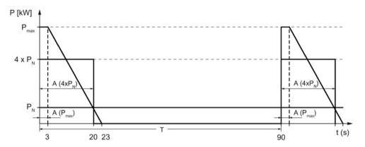
Figure 7-7 Duty cycles for braking resistors with a thermostatic switch
