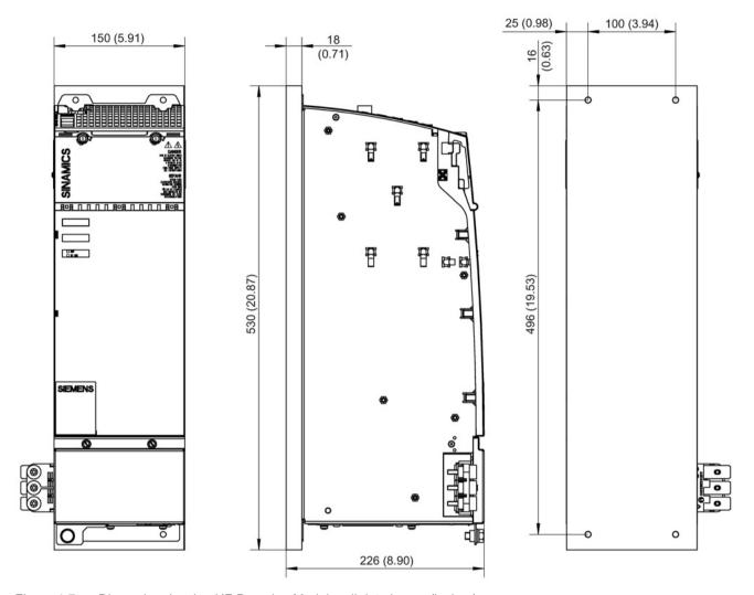
Figure 4-7 Dimension drawing HF Damping Module, all data in mm (inches)
