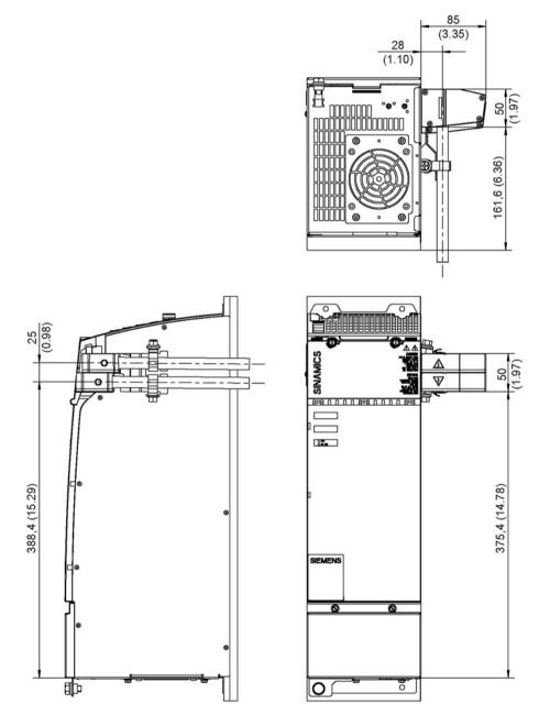
Figure 9-2 Dimension drawing of the HF Damping Module with DC link adapter, all dimensions in mm and (inches)
