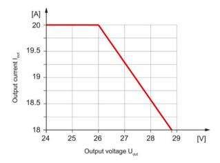
Figure 8-6 Current derating for ambient temperatures >40 °C as a function of the output voltage
