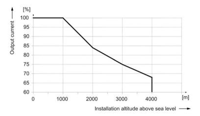
Figure 4-26 Output current as a function of the installation altitude
