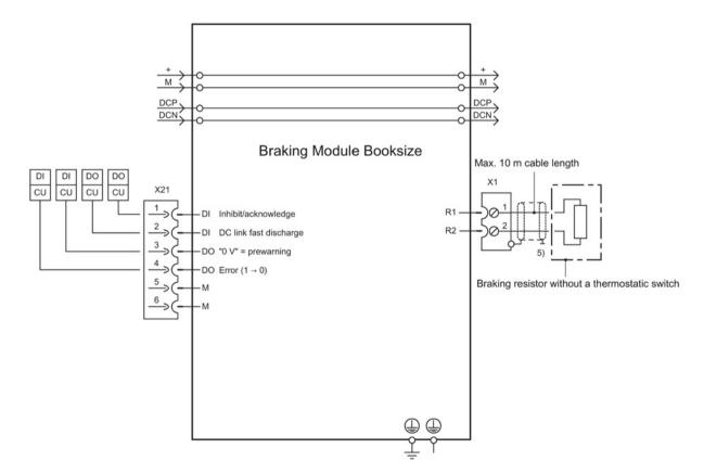
Figure 6-2 Connection example of a Braking Module Booksize
