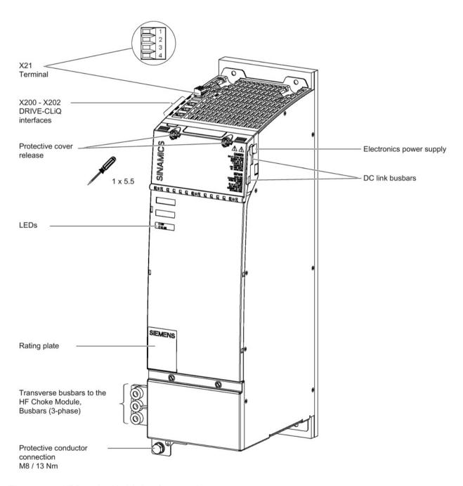
Figure 4-5 HF Damping Module interface overview
