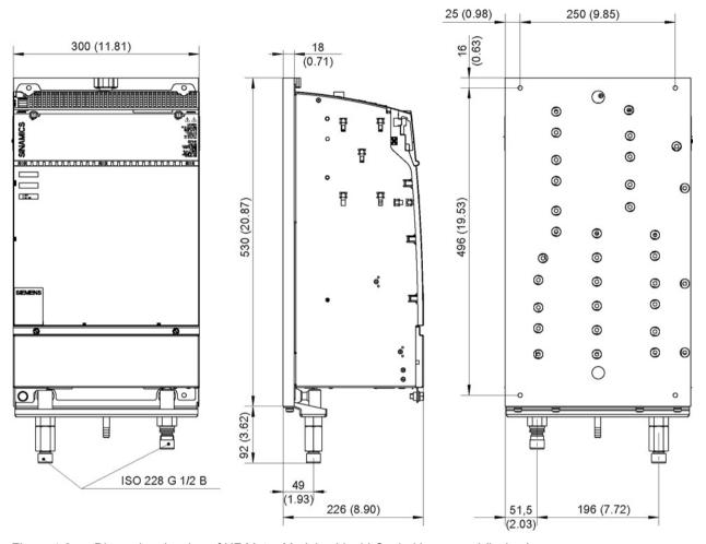
Figure 4-3 Dimension drawing of HF Motor Modules Liquid Cooled in mm and (inches)
