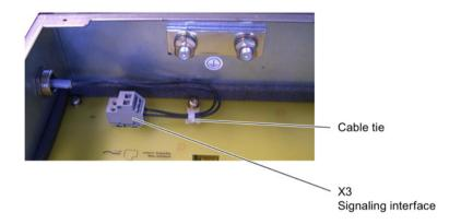
Figure 5-7 Connecting terminal X3 of the Voltage Protection Module
