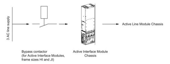
Figure 3-2 Block diagram, line connection, chassis
