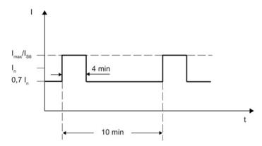
Figure 4-23 S6 duty cycle with initial load with a duty cycle duration of 600 s
