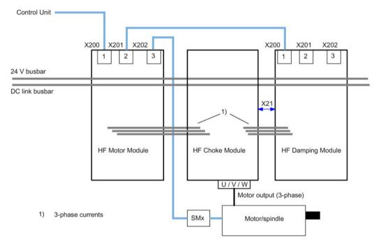
Figure 10-1 DRIVE-CLiQ topology at the High Frequency Drive (16 kHz)
