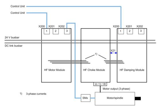
Figure 10-2 DRIVE-CLiQ topology at the High Frequency Drive (32 kHz)
