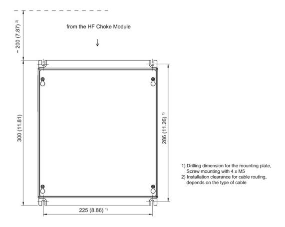
Figure 5-6 Mounting dimensions for a Voltage Protection Module VPM 200 Dynamik
