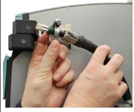
1. Fix the first core of the DC link connecting cable to the profile rail using a cable clamp.
