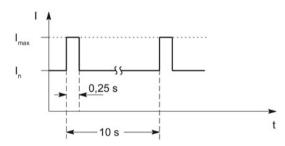
Figure 4-21 Load cycle with previous load
