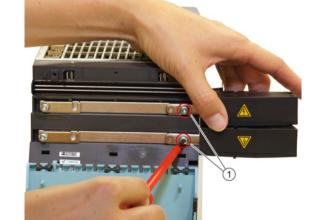
3. Fix the DC link adapter (1.8 Nm) using the previously removed DC link screws. Use the **right-hand** holes ①.
