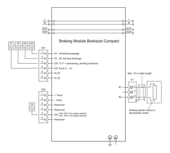
Figure 6-7 Connection example for Braking Module Booksize Compact and braking resistor without a thermostatic switch
