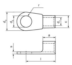
Figure 11-1 Dimension drawing of cable lugs
