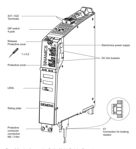
Figure 6-6 Interface overview, Braking Module Booksize Compact
