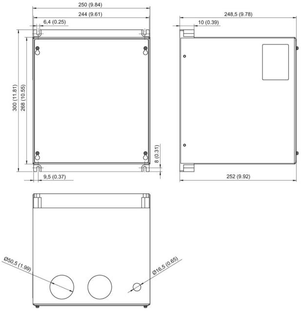
Figure 5-5 Dimension drawing of the Voltage Protection Module VPM 200 Dynamik, all data in mm (inches)
