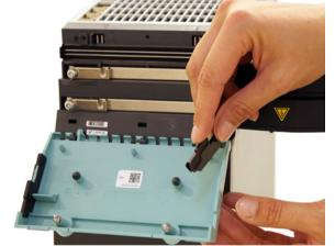
4. Remove the DC link side cover and close the protective cover until you hear it engage.
