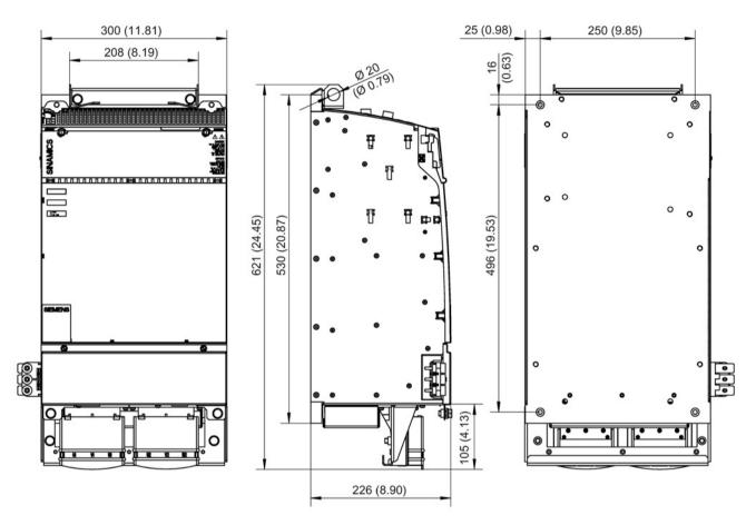
Figure 4-6 Dimension drawing HF Choke Module, all data in in mm (inches)
