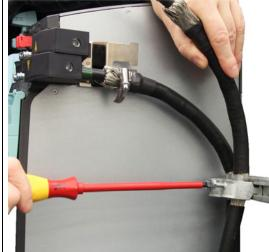
5. Tighten the screw of the hose clamp using a suitable screwdriver.
