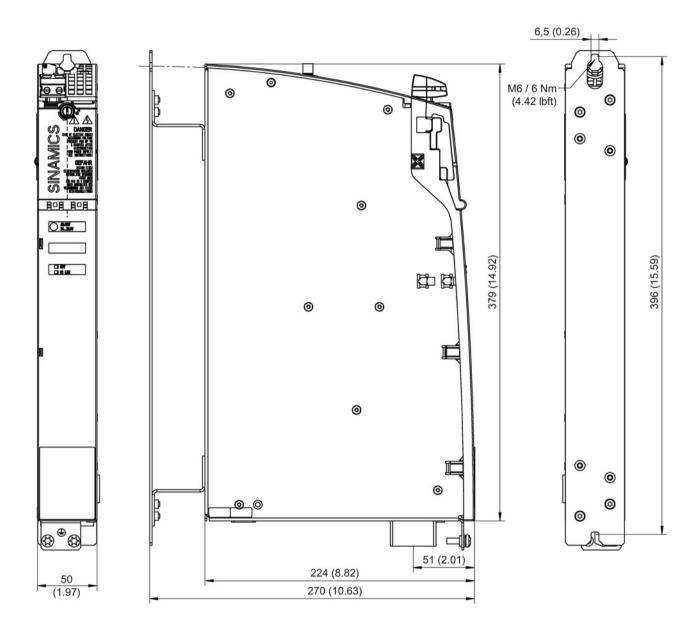
Figure 8-4 Dimension Control Supply Module, all dimensions in mm and (inches)
