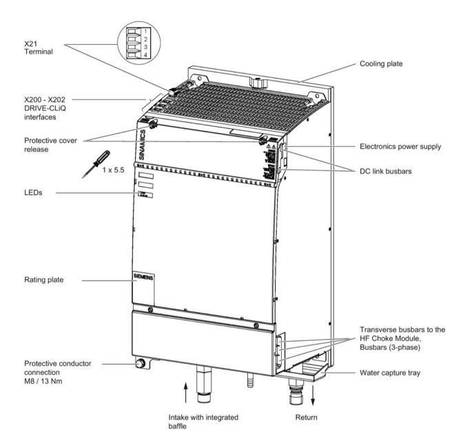
Figure 4-2 Interface overview of HF Motor Modules Liquid Cooled
