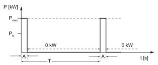
Figure 6-12 Duty cycle for braking resistors without a thermostatic switch
