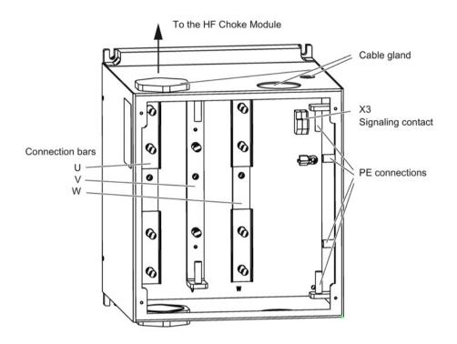
Figure 5-1 Interface overview, Voltage Protection Module VPM200 Dynamic (without cover)
