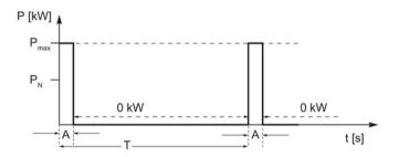
Figure 7-6 Duty cycle for braking resistors without a thermostatic switch
