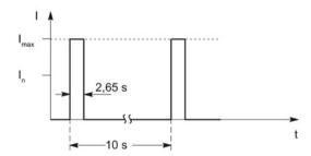
Figure 4-22 Load cycle without previous load
