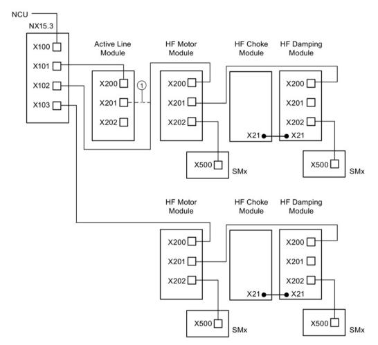
(1) For operation with only one HF Drive 16 kHz, the DRIVE-CLiQ cable can be directly connected from the Active Line Module to the HF Motor Module.
