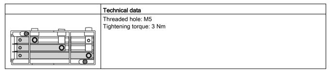
Table 4- 14 Busbars to the HF Damping Module
