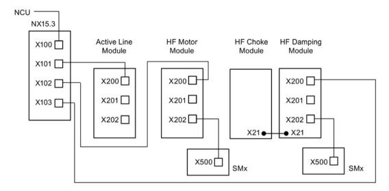
Figure 10-4 DRIVE-CLiQ topology for one HF Drive 32 kHz (31.25 μs) with Active Line Module and NX module
