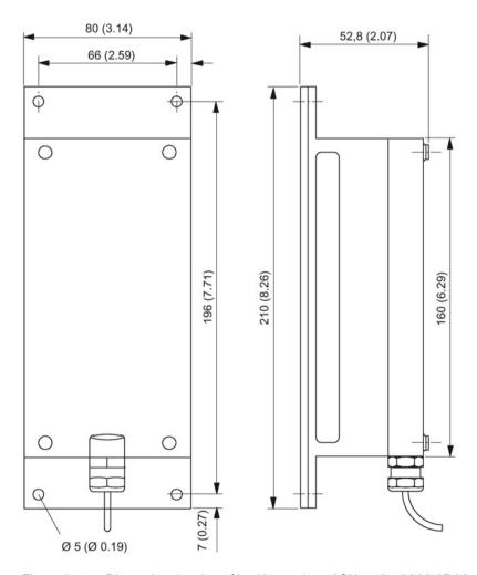
Figure 7-1 Dimension drawing of braking resistor 6SN1113-1AA00-0DA0 where  $P_n/P_{max} = 0.3 \text{ kW}/25 \text{ kW}$ , all dimensions in mm and (inches)
