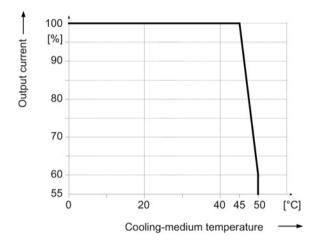
Figure 4-27 Output current as a function of the coolant temperature
