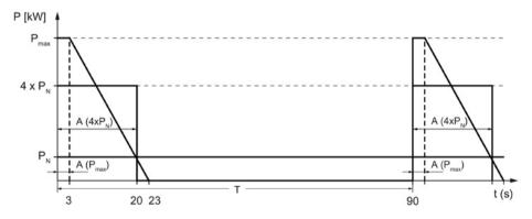
Figure 6-13 Duty cycles for braking resistors with a thermostatic switch
