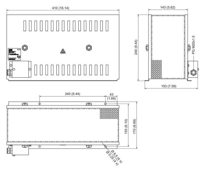
Figure 7-2 Dimension drawing of braking resistor 6SL3100-1BE31-0AA0 where  $P_n/P_{max}$  = 1.5 kW/100 kW, all dimensions in mm and (inches)
