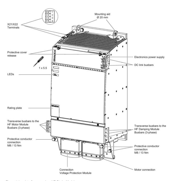
Figure 4-4 Interface overview, HF Choke Module
