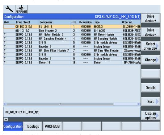
Figure 10-5 High Frequency Drive in the configuration view
