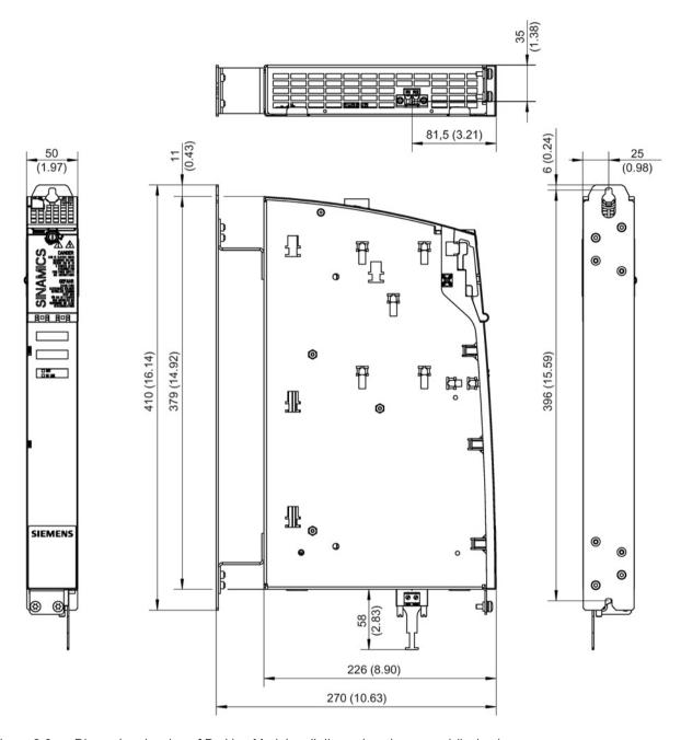
Figure 6-3 Dimension drawing of Braking Module, all dimensions in mm and (inches)
