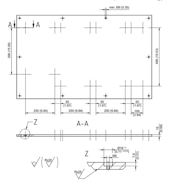
Figure 4-9 Drilling pattern for the High Frequency Drive with Active Line Module booksize, all data in mm and (inches)
