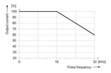
Figure 4-28 Output current as a function of the pulse frequency for a 225 A HF drive
