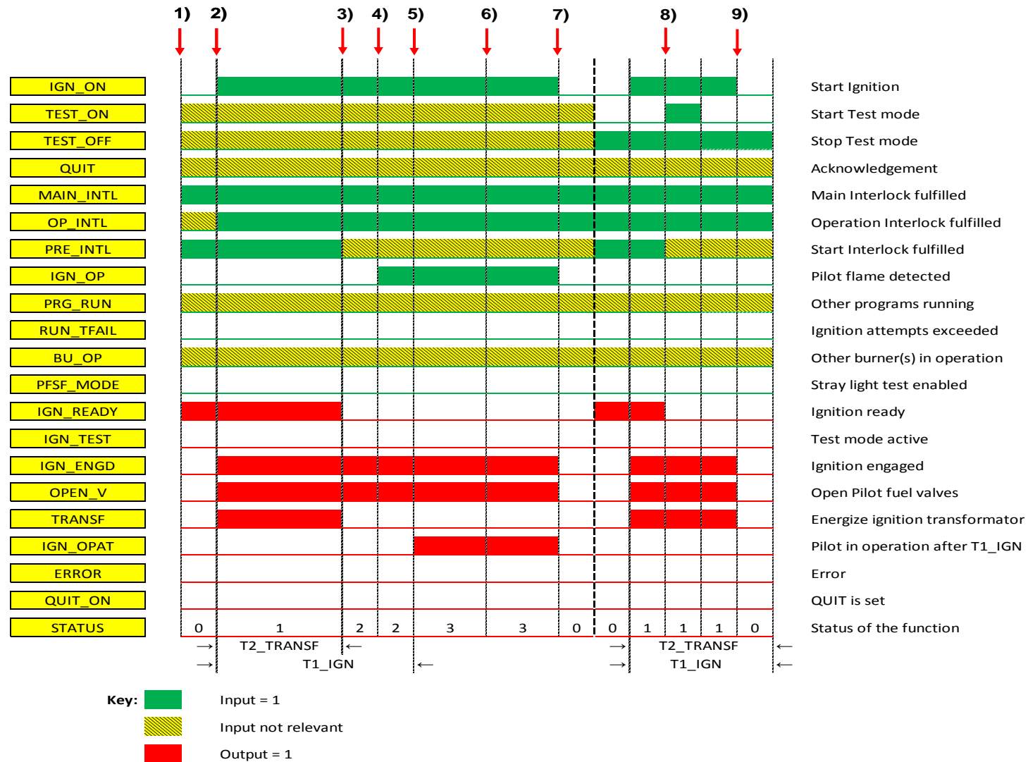
Figure 3-17 Time diagram of the function F_IGNTR in normal operation
