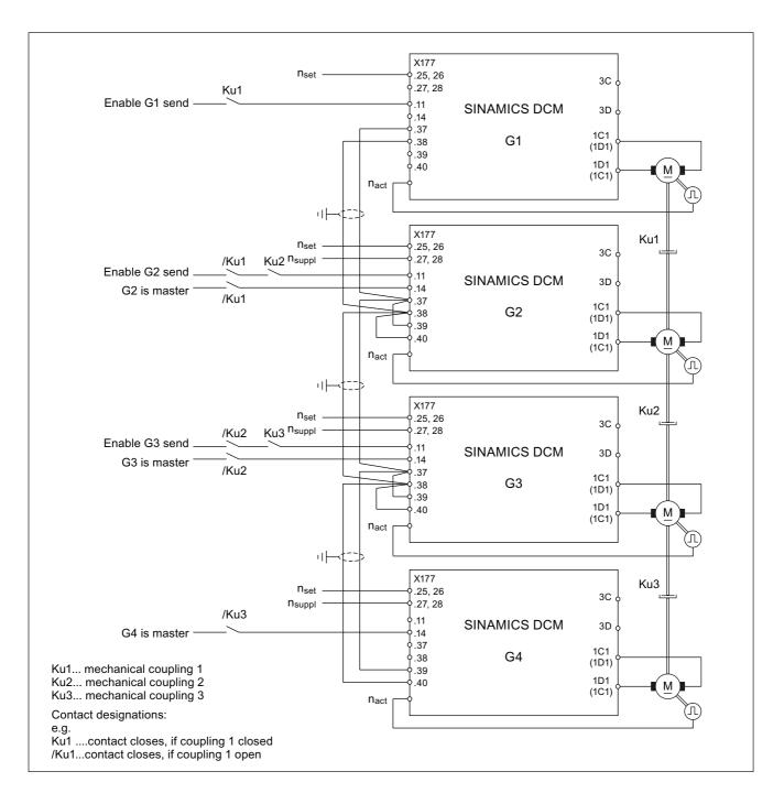
Due to the feedback signals of the coupling states, in the drive units, the correct marshaling is realized for the peer-to-peer connections. The following table is intended to show this.
