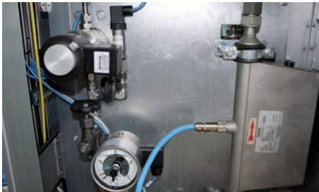
The relatively compact area of Section 1 - Zone 1 is where all Ex equipment (e. g. valves and gas sensors) is located. The major advantage is that the Sitrans FCS200 sensor can be placed in Zone 1 whereas the Siflow FCO70 Ex CT transmitter is placed in Zone 2, allowing the dispenser to utilize less space.
