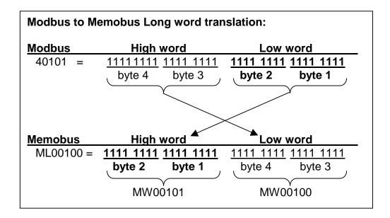
6) Floating point words are 32 bits and are in Intel 486 Single precision format (IEEE Floating Point). The address is expressed in decimal.
